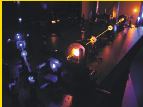
Photograph of a femtosecond synchronously pumped optical parametric oscillator (SPOPO) based on \text{BiB}_3\text{O}_6 emitting in the yellow region of the spectrum. Pumped near 400 nm in the blue by the second harmonic of a Kerr-lens mode-locked Ti:sapphire laser, the SPOPO can generate femtosecond pulses across the full visible range of 480–710 nm, from the blue-green, through to yellow, orange and red.
