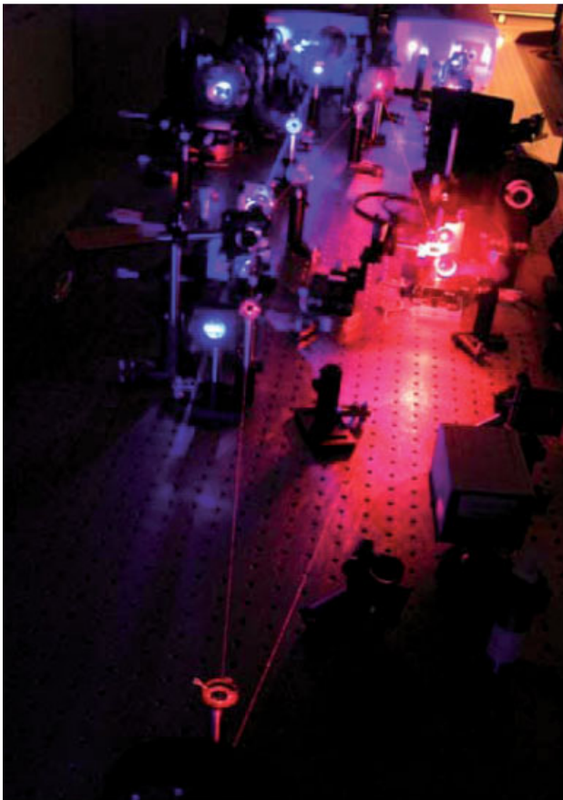
Figure 36 (online color at: www.lpr-journal.org ) Photograph of the blue-pumped BIBO femtosecond SPOPO oscillating in the red, with intracavity frequency doubling in BBO to provide output pulses in the UV.
