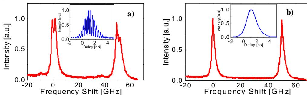
Fig. 4. Interferogram and temporal pulse shape (inset): a) without optical feedback; b) with optical feedback.
