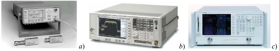
Figure 4. Basic measurement equipment: a) wattmeter W; b) spectrum analyser SA; c) network analyser NA
