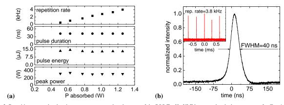
Fig. 2. Repetition rate, pulse duration, output energy and peak power of the PQS Tm,Ho:YLF laser vs. absorbed pump power for  $T_{\rm OC}$ =1.5% (a) and Q-switched pulse shape and pulse train (inset) (b).
