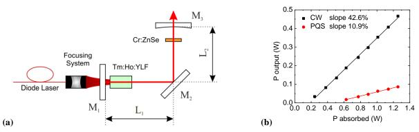
Fig. 1. (a) Setup of the PQS  $Tm_1Ho:YLF$  laser.  $M_1:$  dichroic pump mirror,  $M_2:$  HR-laser, HT-pump mirror,  $M_3:$  output coupler. (b) Output power vs. absorbed pump power for 5.8% OC in CW and PQS regimes.
