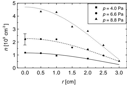
Fig. 4. Radial profiles of the plasma density ( $n$ ) at  $B_0 = 0.065$  T and different values of the gas pressure  $p$ . The fits of the experimental data are with Bessel-type of density profiles according to the least-square method.
