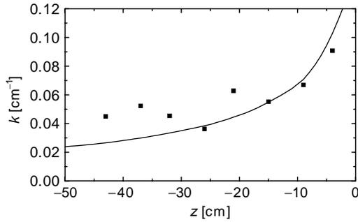
Fig. 2. Measured axial ( $z$ ) variation (symbols) of the wave-number ( $k$ ) at  $p = 4.0$  Pa and  $B_0 = 0.081$  T and comparison with a theoretical result (full curve) taken from the wave phase diagram of the azimuthally symmetric Travelpiece–Gould mode of radially inhomogeneous collisional plasma column.
