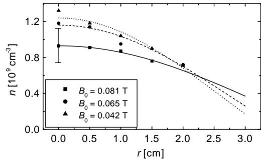
Fig. 5. Radial profiles of the plasma density ( $n$ ) at  $p = 4.0$  Pa and different values of the external magnetic field. The fits of the experimental data are with Bessel-type of density profiles according to the least-square method.
