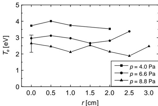
Fig. 3. Radial profiles of the electron temperature ( $T_e$ ) at  $B_0 = 0.065$  T and different values of the gas pressure  $p$ .
