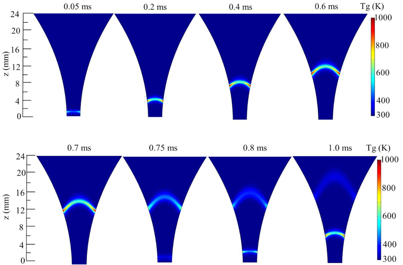
**Figure 6.** Time and spatial evolution of the gas temperature in the  $yz$  plane, at a current of 28 mA and a gas flow rate of  $101 \text{ min}^{-1}$ .
