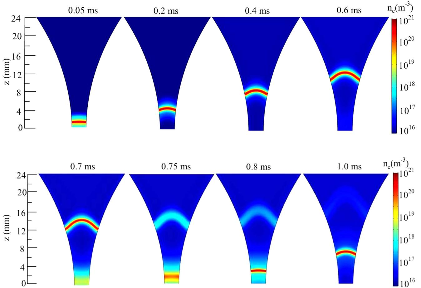
**Figure 8.** Time and spatial evolution of the electron density in the  $yz$  plane, at a current of 28 mA and a gas flow rate of  $101 \text{ min}^{-1}$ .
