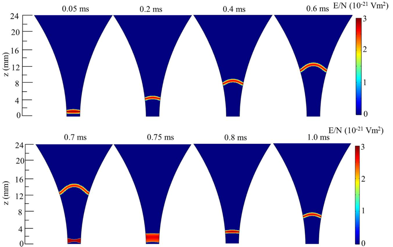
**Figure 5.** Time and spatial evolution of the reduced electric field in the  $yz$  plane, at a current of 28 mA and a gas flow rate of  $101 \text{ min}^{-1}$ .
