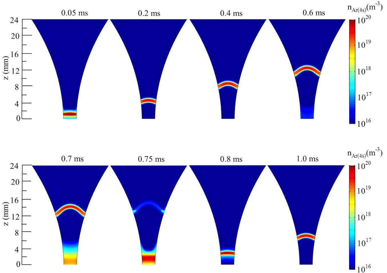
**Figure 12.** Time and spatial evolution of the Ar(4s) excited state density in the  $yz$  plane, at a current of 28 mA and a gas flow rate of  $101 \text{ min}^{-1}$ .
