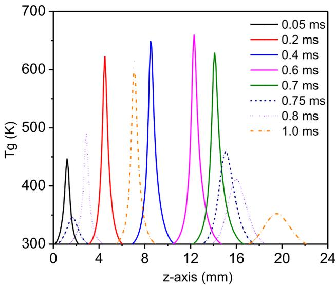
**Figure 7.** Distribution of gas temperature along the  $z$ -axis at different times, for a current of 28 mA and a gas flow rate of  $101 \text{ min}^{-1}$ .
