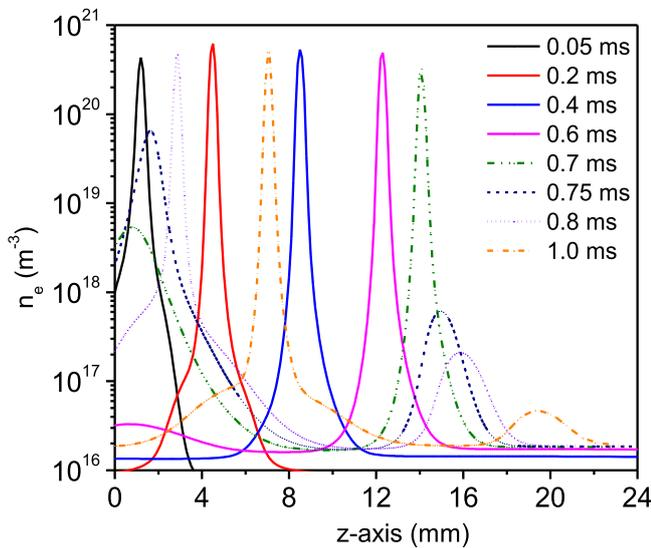
**Figure 9.** Distribution of electron density along the  $z$ -axis at different times, for a current of 28 mA and a gas flow rate of  $101 \text{ min}^{-1}$ .
