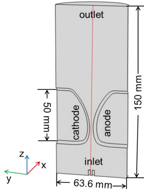
**Figure 1.** 3D Cartesian geometry used in the model. The zero of the  $z$ -axis in the figures below is at the position of the shortest interelectrode gap, which is 43 mm from the position of the gas nozzle (gas inlet).
