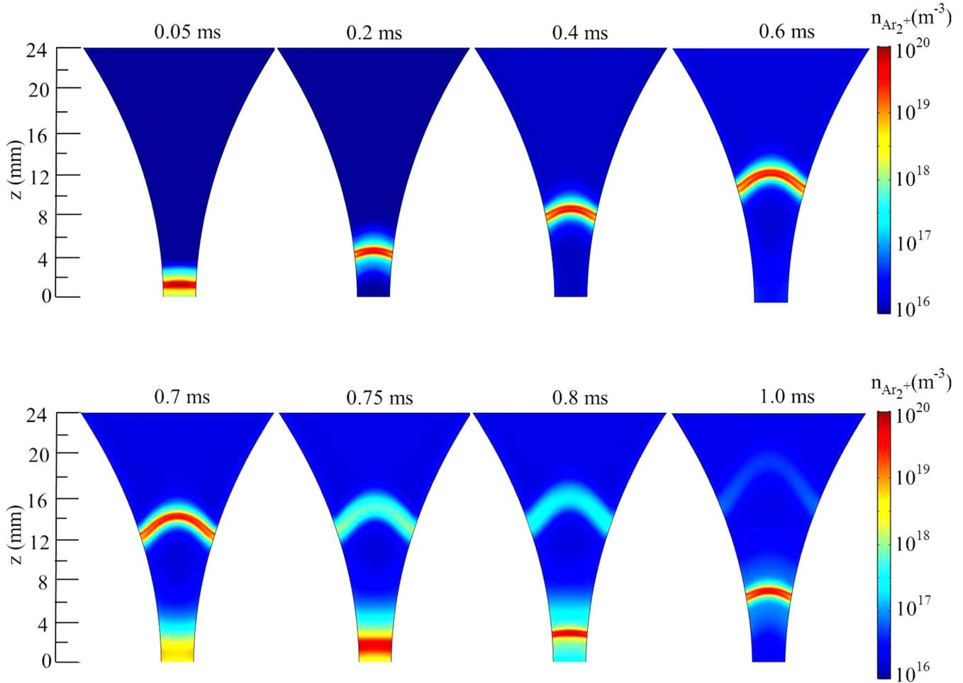
**Figure 11.** Time and spatial evolution of the  $\text{Ar}_2^+$  ion density in the  $yz$  plane, at a current of 28 mA and a gas flow rate of  $101 \text{ min}^{-1}$ .
