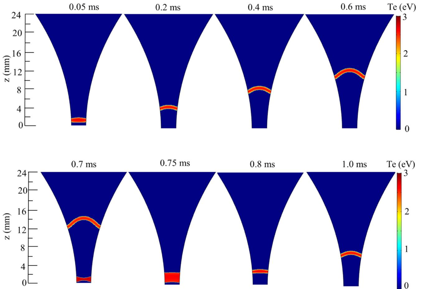
**Figure 4.** Time and spatial evolution of the electron temperature in the  $yz$  plane, at a current of 28 mA and a gas flow rate of  $101 \text{ min}^{-1}$ .
