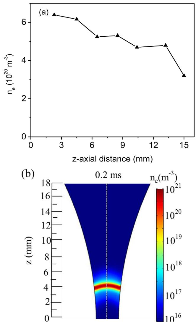
**Figure 3.** Calculated maximum electron density (in the center of the arc) along the  $z$  axis, as a function of distance from the shortest interelectrode gap (a), and illustration of the electron density distribution in the  $yz$  plane (b), for a current of 28 mA and a gas flow rate of  $10 \text{ l min}^{-1}$ .
