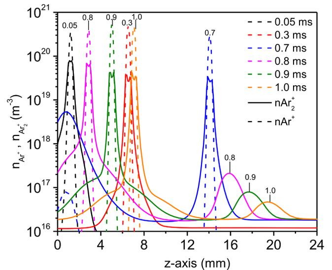
**Figure 10.** Distribution of  $\text{Ar}^+$  (dashed lines) and  $\text{Ar}_2^+$  (solid lines) ion density along the  $z$ -axis at different times, for a current of 28 mA and a gas flow rate of  $101 \text{ min}^{-1}$ .
