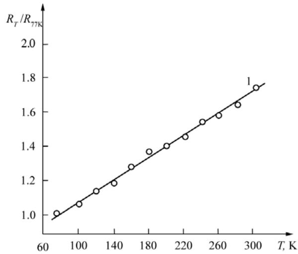
**Fig. 3.** Temperature dependence of Hall coefficient ( $x = 0.002$ ,  $y = 0.005$ )
