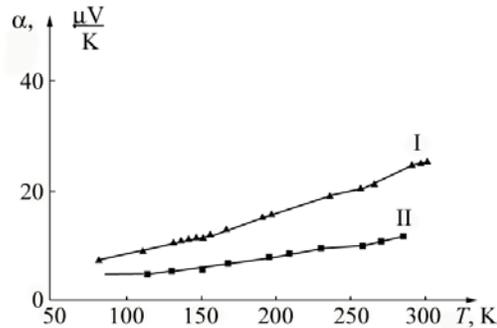
**Fig. 1.** Temperature dependence of thermoelectric power for samples  $[\text{Pb}_{1-x}\text{Bi}_x]_{1-y}\text{Gd}_y\text{Te}$  doping with Bi: I)  $x = 0.002$  ; II)  $x = 0.003$
