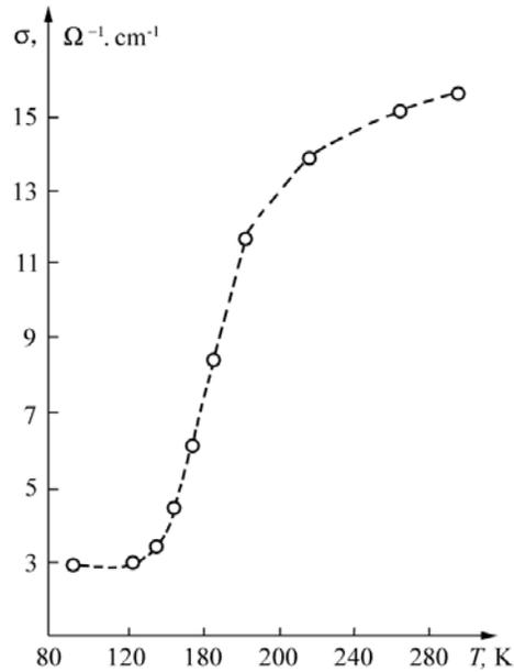
**Fig. 2.** Temperature dependence of electroconductivity for sample  $[\text{Pb}_{1-x}\text{Bi}_x]_{1-y}\text{Gd}_y\text{Te}$  with  $x = 0.001$
