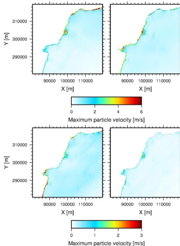
**Fig. 5.** Computed field of maximum particle velocity: ShablaNE-SW (upper left), ShablaW-E (upper right), Balchik (bottom left), NW Turkey (bottom right) scenarios
