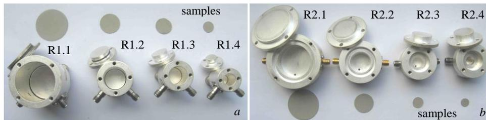
**Fig. 2.4.** Pairs of optimized measurement resonators with different diameters: *a)* TE-mode R1 (30, 18, 15, 10 mm) and *b)* TE-mode R2 (30, 18, 10, 8 mm), which cover frequency range 5-39 GHz
