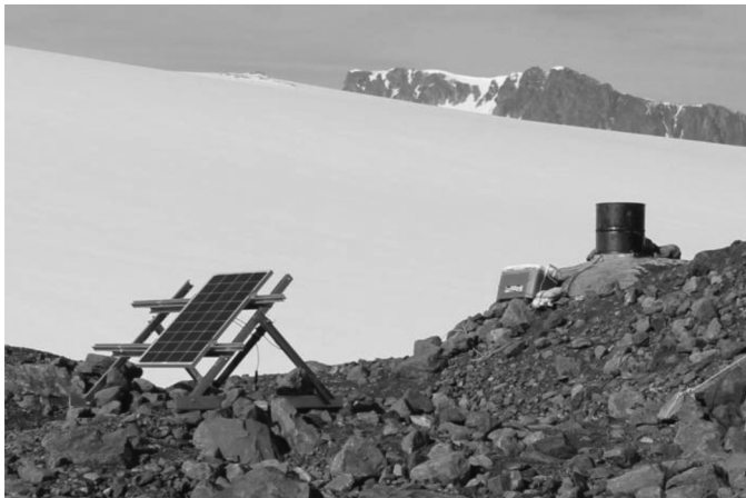
Fig. 3. Seismological equipment installed on the pillar and solar panel
