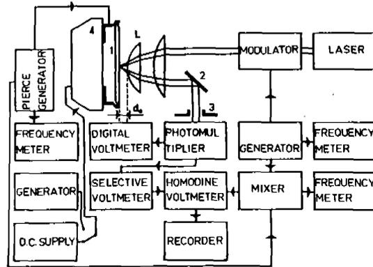
Fig. 1. Block-diagram of the experimental equipment: 1-quartz plate, 2-mirror, 3-mask, 4-telephone membrane.
