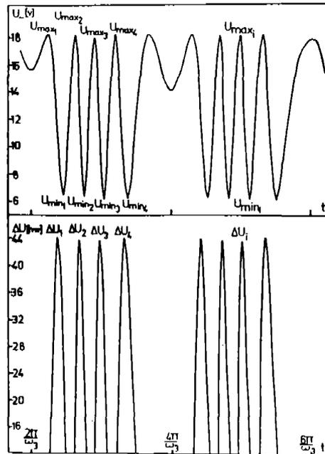
Fig. 3. Recorder registration of the voltages  $u_{\sim i}$  and  $\Delta u_i$  used for calculation of the amplitude of vibrations  $d'_o$  for one point on the surface of the quartz plate.
